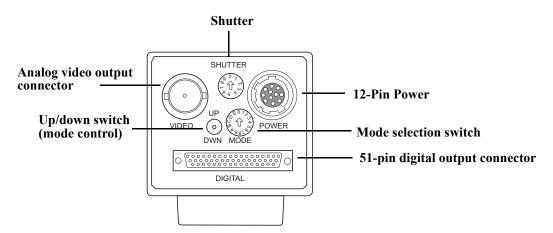
FIGURE 9. Rear Panel Layout (TM-6710CL)
